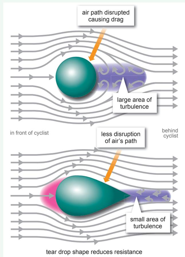
the teardrop shaped frame. Brake and gear cables can create drag if they are hanging or loose so bike manufacturers tend to hide these behind the frame to reduce drag. The human head is a block shape that increases the frontal area of the cyclist. By wearing an **aerohat** (teardrop shaped helmet), drag is reduced as it cuts through the air and reduces the pressure differences which can occur.
